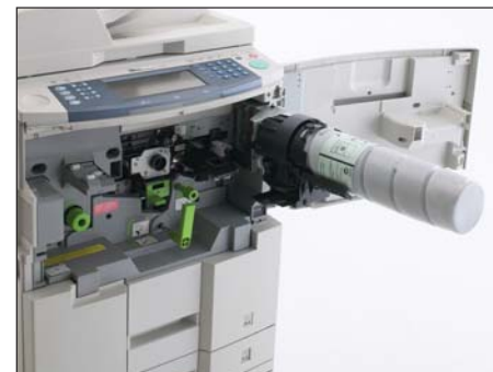
Changing the toner bottle is as easy as opening the front panel door.
